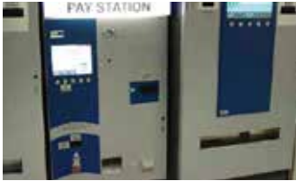
Picture 2.8.1. Sample of parking ticket machines at two different heights
