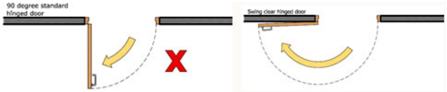
Picture 5.7.3.1. Opening and closing of door with multiple hinges
