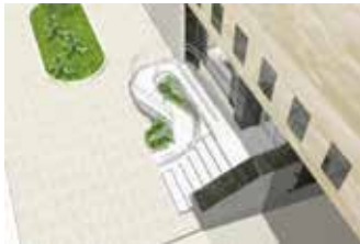
Picture 1.2.1.5. Modifying ramp for a narrow area
